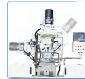
Swivelable mill head from -90° to +90° allows for various operations. pneumatic tool clamping as optional.
