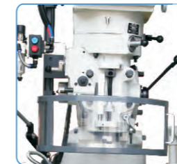
Spindle feed by hand or automatic (0.04/0.08/0.15mm/r)
