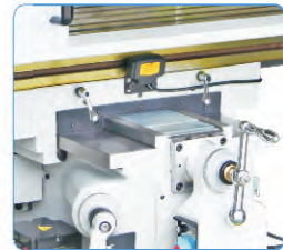
Rectangular guideway in Y and Z-axis.
