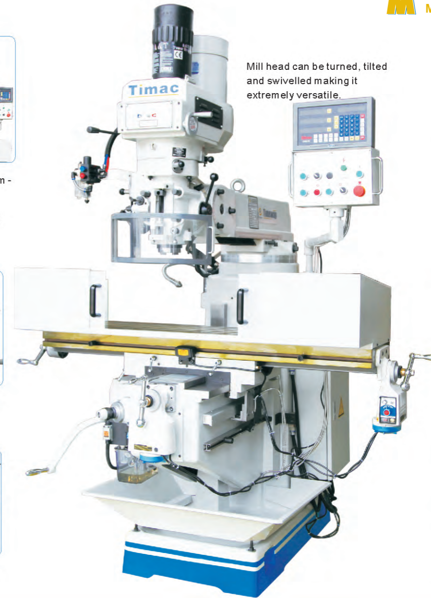
Spindle feed by hand or automatic (0.04/0.08/0.15mm/r)
