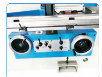
The longitudinal movement of the worktable is driven by hydraulic or by handwheel. The worktable can rotate to a certain degree so as to be suitable for grinding taper. The wheelhead cross feed is driven by hydraulic, which realizes automatic periodical feed and rapid feed. It can also do rough and fine feed through handwheel.
