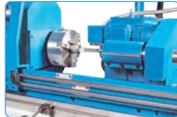
Grinding head can be rotated 180° to change from inside to outside grinding.
