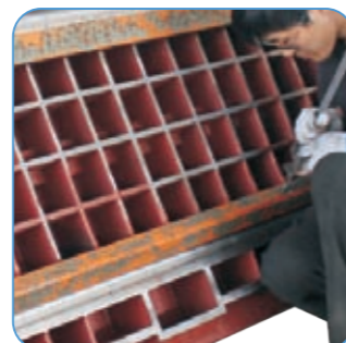
The guideway is coated with Turcite and precision hand scraped, move smoothly and keep the accuracy long life.
