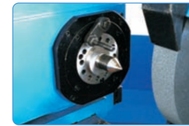
Grinding spindle with segmented high-precision bearings, adjustable and low maintenance. Grinding spindle adopts oil-bath lubrication and coolant (N2 oil). Workhead spindle speeds are infinitely variable and driven frequency motor and interver, can be easily adjusted and optimized during the machining process.
