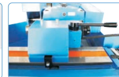
Standard tailstock can operate either manual by handle or hydraulic control by foot pedal, sometime hand wheel on the end of tailstock can adjustable clamping force.
