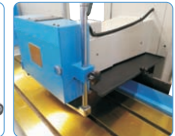
Precision grinding spindle runs in maintenance-free, support by preload high precision angular ball bearing. Super great power spindle unit is most important to the machine. It is really an elaboration under well designed, and our ultimate goal is to balance high rigidity and great accuracy.
