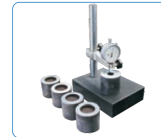
Precision grinding 5pcs test parts (diameter 50mm, 45#steel, equal thickness tolerance 0.005/300mm).
