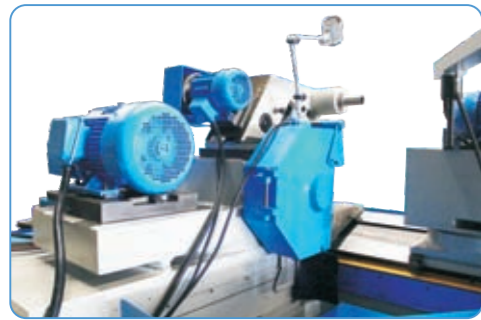
The workhead spindle, wheelhead spindle, internal grinding spindle are driven by separate motors.
