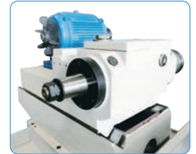
Wheelhead spindle is supported by bimetal shell bearing, which make the spindle have high rigidity and stability, ensure heavy, excellent finishing surface.
