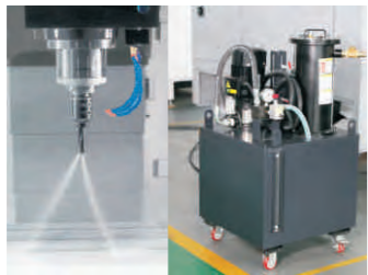
Coolant through spindle center Coolant to be supplied to the tip through the holes of the spindle and tool.
