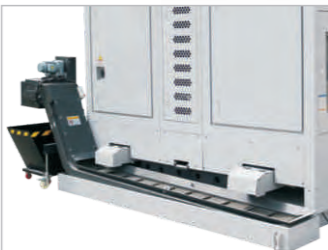
Chip conveyor Reduced chip accumulation inside the machine and operator spends less time removing chips.
