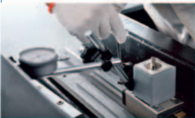
06/ 齿条安装 Rack installation
